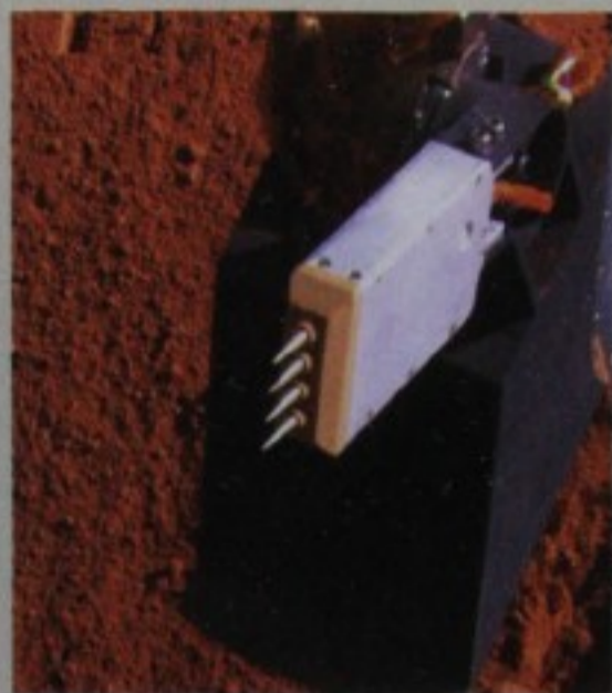
In early September, NASA's Phoenix Lander inserted the four needles of its thermal and electrical conductivity probe into the ground for a full Martian day, or sol, to measure changes in the soil from day to night.
