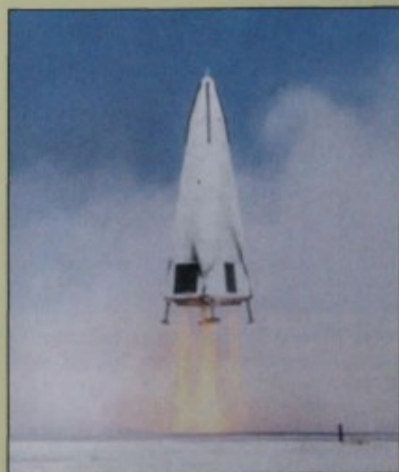
All four of the DC-XA's landing gear extended properly at the end of this flight in June. But the rocket fell over and burned the following month when it touched down on only three legs. Courtesy NASA.
