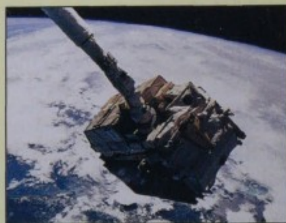
Plucked from space after 11 months in orbit, the European Retrievable Carrier dangles from the Space Shuttle Endeavour 's robot arm. Courtesy NASA.
