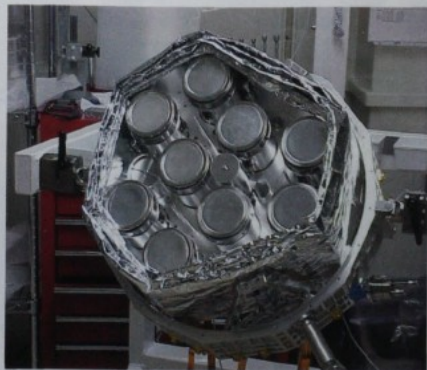
Left: From its 600-kilometer-high orbit, the High Energy Solar Spectroscopic Imager (HESSI) will monitor the Sun's powerful flares. Right: The business end of HESSI consists of these nine germanium detectors, which determine the energies of X- and gamma rays in solar flares. In space the detectors are being chilled to about 75° Kelvin (-324°F). Courtesy NASA/Goddard Space Flight Center.
