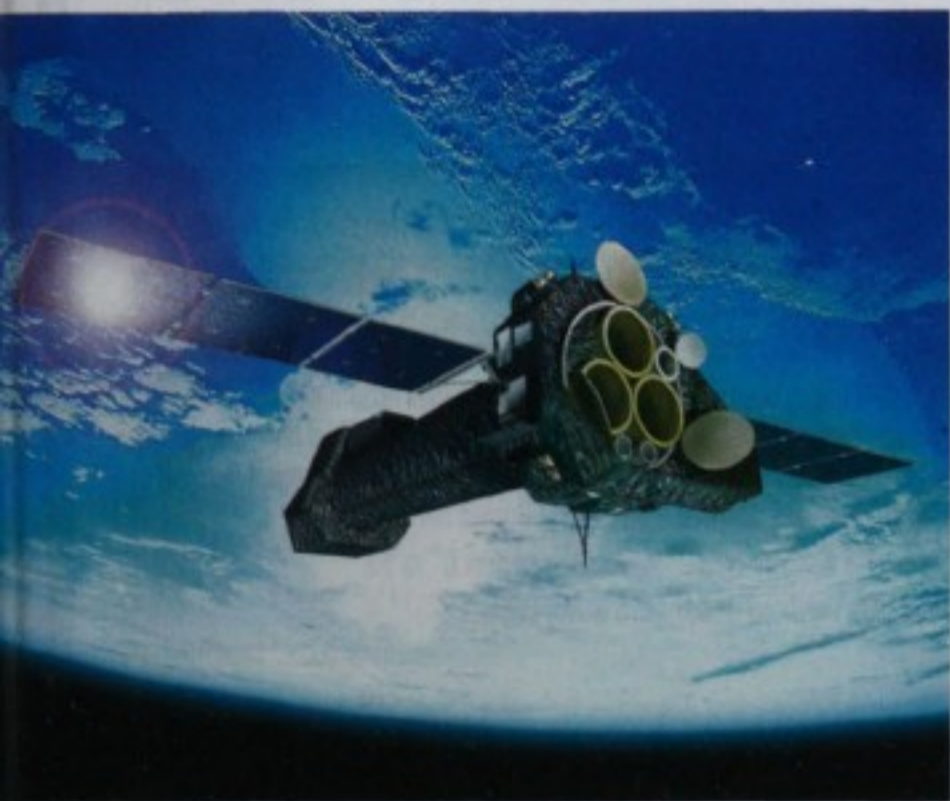
The X-ray Multi-mirror Mission observatory is depicted looping near Earth at the perigee of its 850-by-114,000-kilometer orbit. The 3.9-ton spacecraft is the largest scientific satellite yet developed by the European Space Agency. Courtesy ESA.
