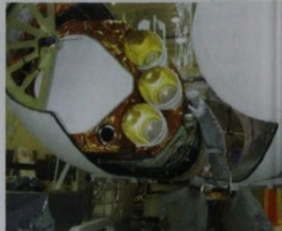
Technicians install an aerodynamic fairing around the SWAS spacecraft two weeks before its December launch aboard a Pegasus XL rocket.
