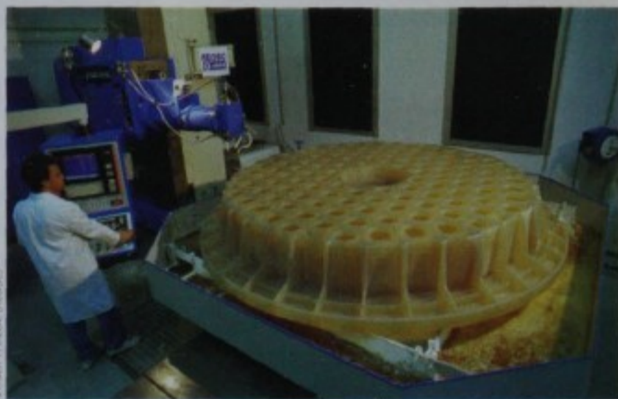
This "lightweight" 2.7-meter-wide disk of glass, weighing nearly a ton, is destined to be the primary mirror for a flying observatory called SOFIA.
