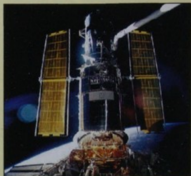
During its December 1993 servicing by shuttle astronauts, the Hubble Space Telescope received the new pair of solar-cell "wings" shown above. These flexible blankets will in turn be replaced by rigid panels during the shuttle visit now planned for 1999. Courtesy NASA.
