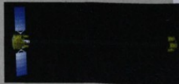
NASA's NuSTAR satellite will carry three high-resolution X-ray telescopes having very long focal lengths.
