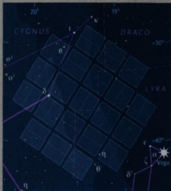
The Kepler spacecraft will stare at this field between Vega and the western wing of Cygnus, monitoring the light from 100,000 stars to find any small planets transiting them. Boxes show the coverage of the camera's CCD chips.
