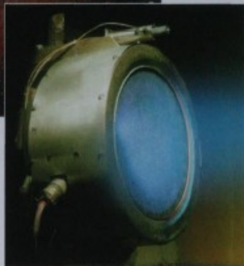
Right: Eerie blue exhaust rushes out of an ion-drive engine at more than 30 kilometers (20 miles) per second. Above: The Dawn spacecraft will use thrusters of this type to reach the asteroids Ceres and Vesta. Courtesy Jet Propulsion Laboratory and William K. Hartmann.
