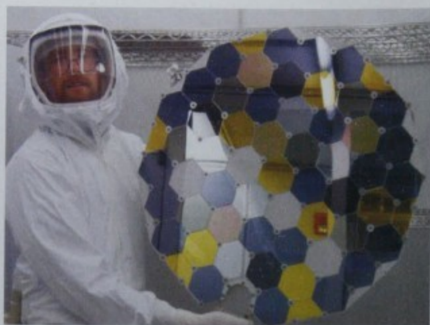
Genesis participant Andy Stone holds one of the spacecraft's five collector arrays in a clean room at the NASA/Johnson Space Center. The hexagonal tiles, each measuring about 10 centimeters across, are made of various materials such as silicon, germanium, artificially grown diamonds, and metallic “glass.”
