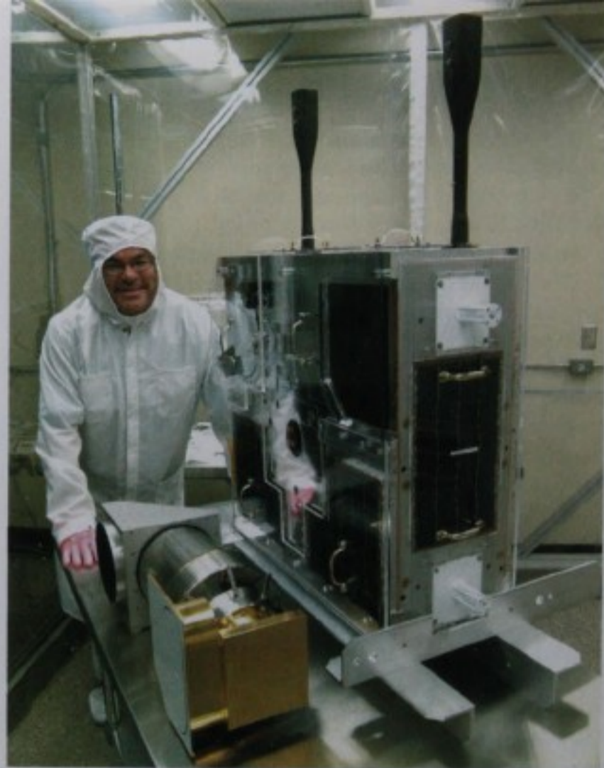
Mission scientist Jaymie Matthews (University of Toronto) checks out the MOST telescope assembly (left foreground) and spacecraft prior to its launch. Courtesy Canadian Space Agency.
