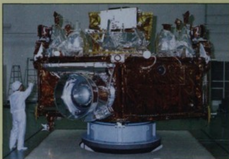
The Infrared Telescope in Space (IRTS) peers from one side of Japan's Space Flyer Unit. A joint Japanese-American instrument, the IRTS surveyed solar-system dust, molecular clouds and the cosmic infrared background during its March-April flight. Courtesy H. Okuda and the Institute of Space and Astronautical Science.
