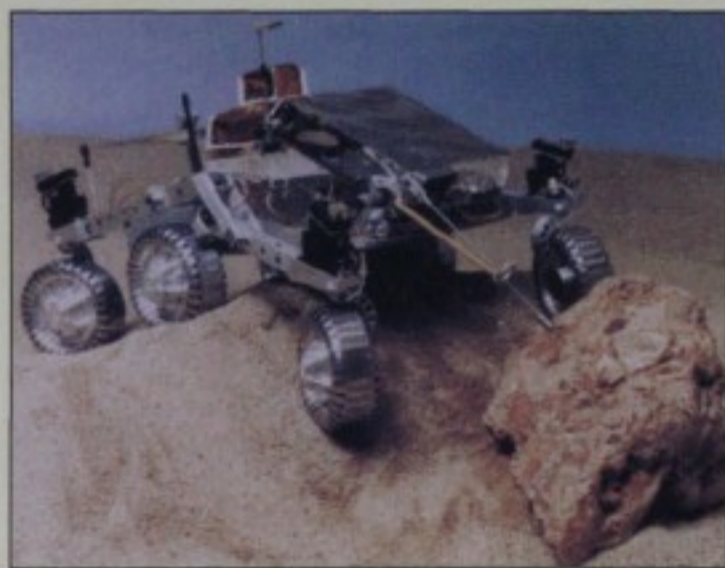
If NASA's Mars Pathfinder successfully lands on the red planet next year after its planned late-1996 launch, it will deploy the Sojourner micro-rover to study Martian rocks and soil. Courtesy the Jet Propulsion Laboratory.
