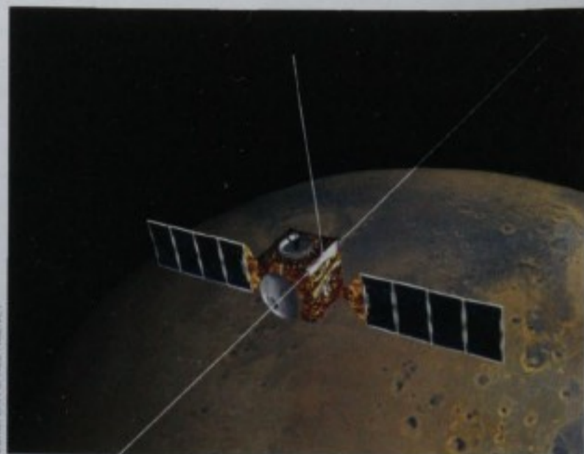
Mars Express carries an extensive suite of instruments, including a ground-penetrating radar system that will employ a 40-meter-long antenna to map buried reservoirs of water.
