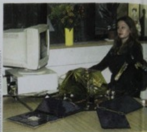
The Mars Express mission will carry an instrumented lander named Beagle 2, seen here as a full-size engineering model.
