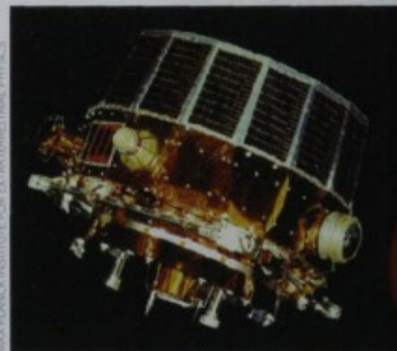
Equator-S carries seven scientific instruments in a spinning, 230-kilogram package measuring 2.3 meters in diameter.
