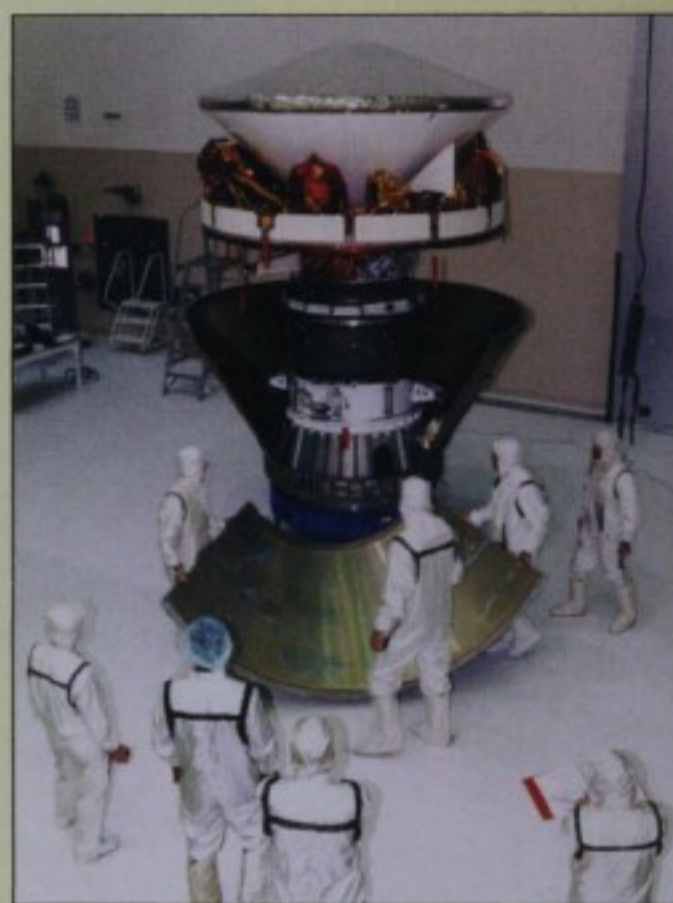
Technicians prepare Mars Pathfinder for its successful December launch at the Kennedy Space Center. The lander and rover are enclosed in the cone-shaped entry module at top. Just below that are the disk-shaped cruise stage and the Delta rocket's upper stage. Courtesy NASA.
