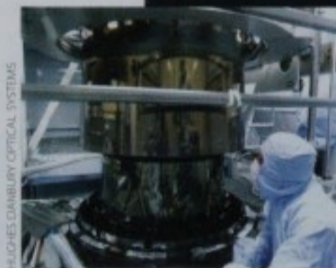
Above. After its launch by the Space Shuttle in September 1998, the Advanced X-ray Astrophysics Facility will ascend to a high orbit for its detailed, sensitive observations of cosmic sources. Left: AXAF's optics are the largest and most accurately shaped X-ray mirrors ever built. When X-rays glance off one of the four nested surfaces, each a precisely tapered cylinder, they are brought to a focus.
