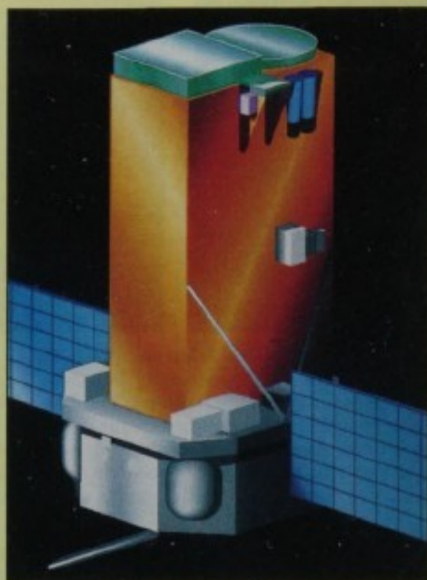
INTEGRAL, the International Gamma-Ray Astrophysics Laboratory, will be launched around 2001 for a two- to five-year investigation of celestial sources of high-energy radiation. Courtesy the European Space Agency.
