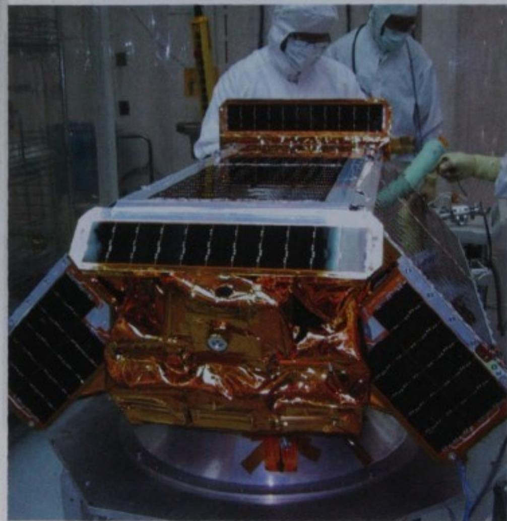
The CHIPS spacecraft sits atop the adapter for the Delta rocket that will launch it into orbit. Six aperture slits for the craft's spectrometer are visible below the small silvery disk in the middle of the gold-colored foil. The black rectangles are solar cells, and the light-blue tube in back, near a hand, is the craft's magnetometer. Courtesy Michael Sholl (Space Sciences Lab, University of California, Berkeley).
