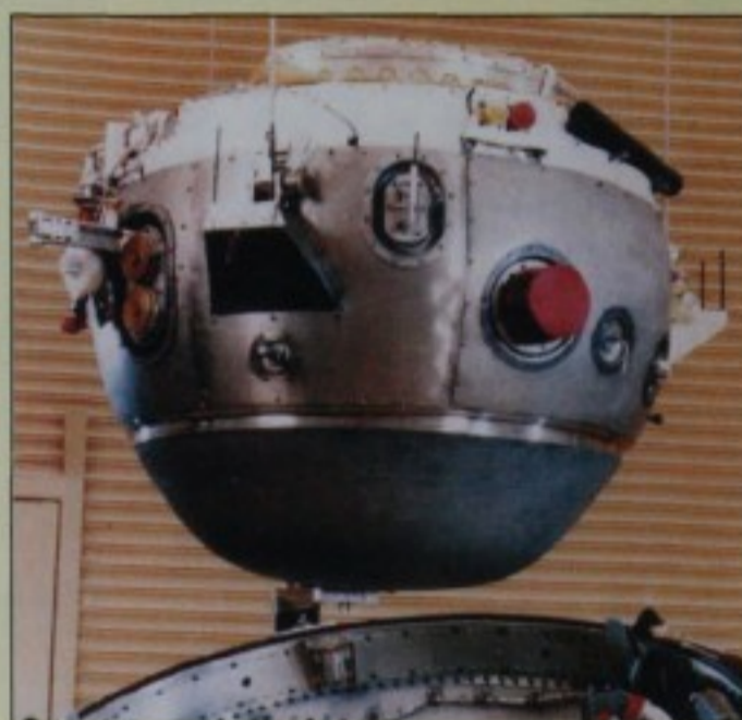
Seen here before launch and without its heat shield, the 1.25-meter Galileo atmospheric probe will plow into Jupiter's cloudtops on December 7th. Courtesy NASA-Ames Research Center.
