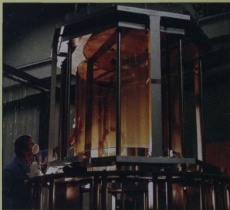
The Advanced X-ray Astrophysics Facility uses nested paraboloidal and hyperboloidal grazing-incidence mirrors, one of which is shown here before getting its reflective coating. Courtesy Hughes Danbury Optical Systems.
