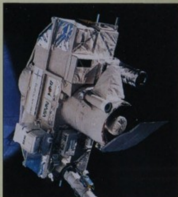
The astronomical shuttle-pallet satellite with its ORFEUS (center) and IMAPS (top right) spectrographs dangles at the end of Discovery 's robotic arm before being set loose for six days last September. Courtesy NASA.
