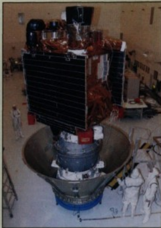
Workers at Kennedy Space Center load Mars Global Surveyor into its payload canister in preparation for its successful launch last November 7th. The gray sphere at bottom is part of the Delta II rocket's upper stage. Courtesy NASA.
