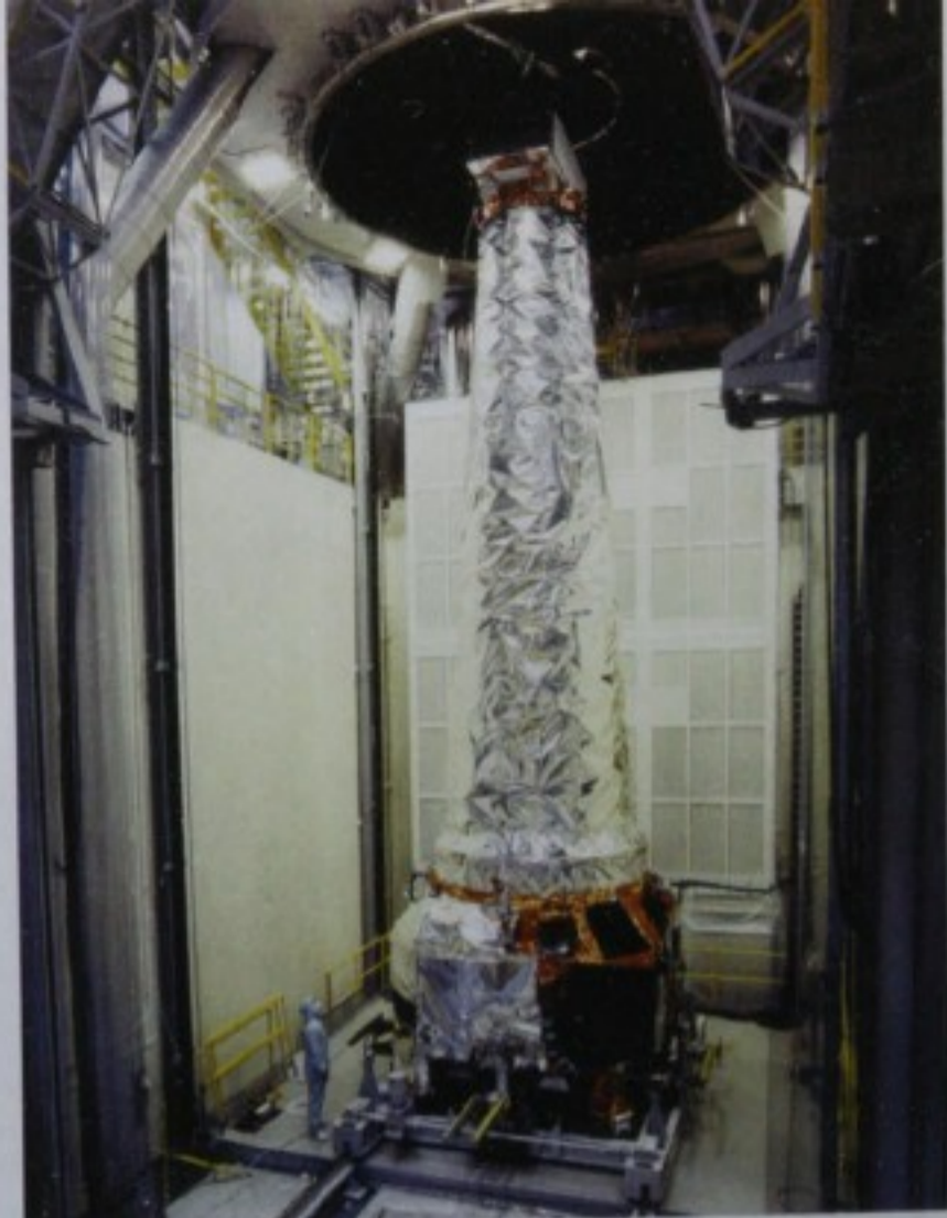
In mid-1998, a year prior to its launch, the Chandra X-ray Observatory was tested to ensure that it could withstand the rigors of space.
