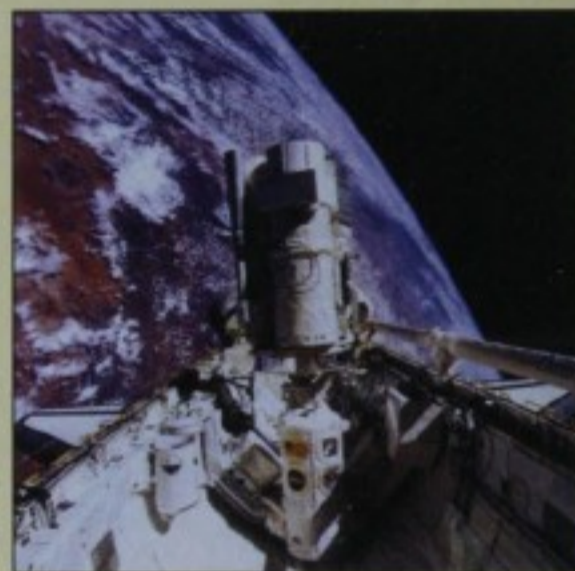
Astro's three ultraviolet telescopes, all on a common mount, peer from the cargo bay of Space Shuttle Endeavour during its historic 16-day flight in March. Courtesy NASA.
