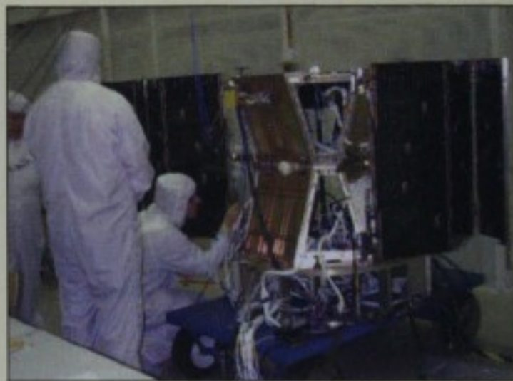
The Submillimeter Wave Astronomy Satellite undergoes a preflight checkout in anticipation of its 1996 launch on a Pegasus XL winged rocket. Courtesy NASA.
