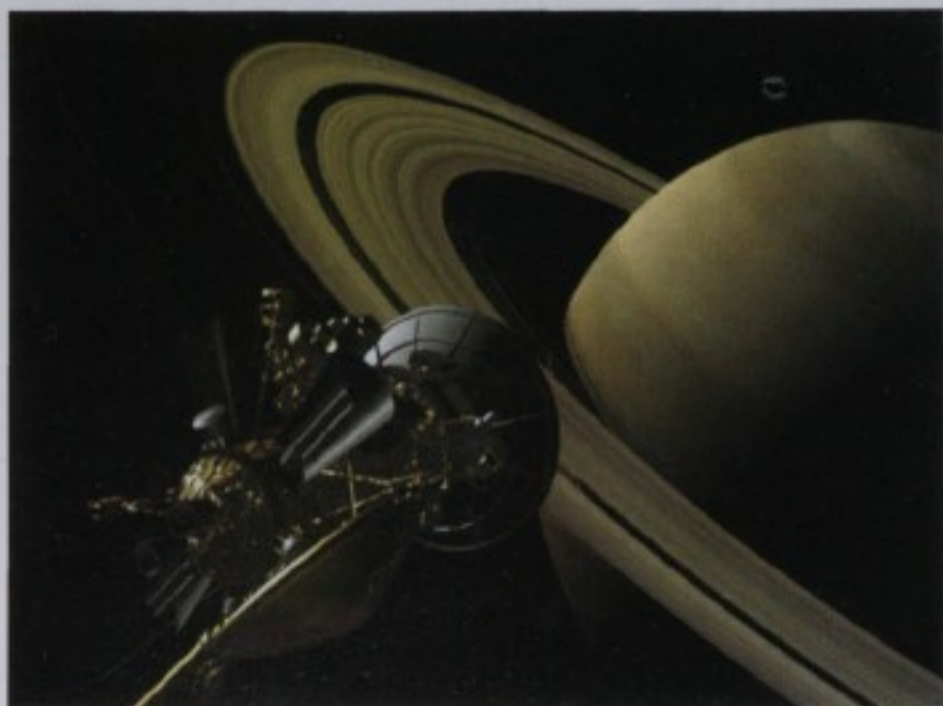
The Cassini probe periodically picks up speed on its way to Saturn through close encounters with other solar-system bodies.
