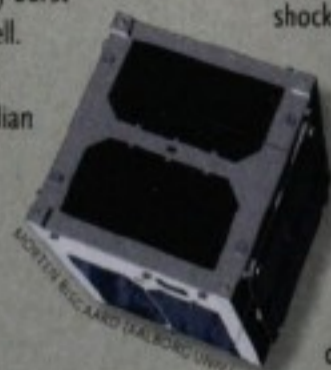
Measuring 4 inches (10 cm) on a side, the high-energy-sensing AAUSat 2 is slightly larger than a softball.
